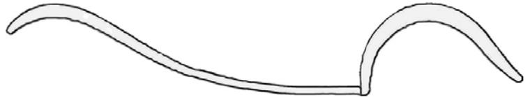
Leave the CS cabin and deck proportions essentially as designed. Stretch the wheelbase by moving the front wheels forward 16 or more inches and fabricate a set of fenders replicating the MG sweep:
