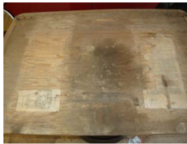
Above, a photo of Gary's M2 seatback, showing the location where the two sheets were installed. Apparently one on each side of the area that tends to get blackened from bits flying off the wearing belts? Note that the lubrication panel goes on the left, opposite how I showed them last issue.
