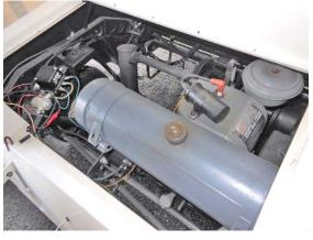
Engine & muffler arrangement.
