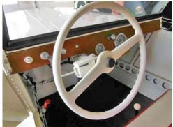
This car has its original hood and dash. Note the smooth curve of the top of the grille, with the crown behind it smoothed back to the center ridge. Hard to replicate. This is also an original dash, made of brown leather-textured hardboard, which deteriorated easily.
