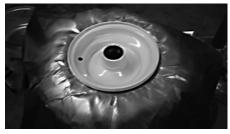
Cut a mask from plastic or heavy paper, with a hole a bit smaller than the wheel diameter. Lay a wheel on a bench and tuck the mask between the portawall and the wheel.
