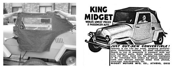
The earliest M2 doors were rather primitive, made of canvas sewn over a wire frame, with plastic windows and not so much as a flap for arm signals. Clearly a temporary fix. As soon as the founders could catch a breath, they worked out something better.
