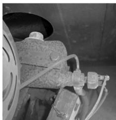
There it is, easy to see and reach from under the car, above the steering box and beside the horn. But you can't get a funnel into it, and if you could, you'd not be able to pour in brake fluid.
