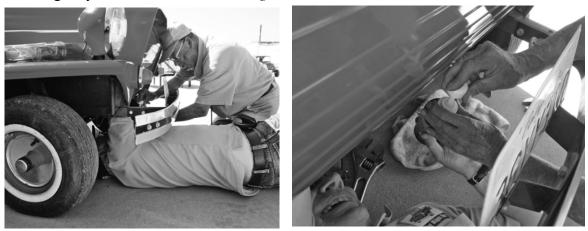
That's me, left, under the front with Gert Gehlhaar supervising? Handing me that big wrench he'd borrowed? No, nothing as simple as that. At right, because the dumb pump won't fit the brake fluid can, it took three hands to fill the master cylinder from below. All because we didn't read Shop Notes to get the right pump!
