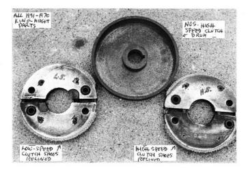
The low-speed and high-speed clutch shoes look almost the same to the untrained eye. The main way to tell the difference is in the distance between the pins that hold the inner springs.
