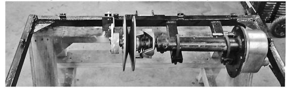
Paul has found that installing a support bearing on the outer end of the shaft makes smoother operation and shifting when starting off. It should also extend the life of the end bearing on the transmission and the whole system.
