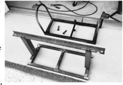
tacked them to the jig. Later, this jig held the pieces in the correct locations while I welded the new assembly together.
