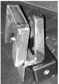
I cut a piece of 1/16" steel plate about the same width as my phone and long enough to hold the clamp
