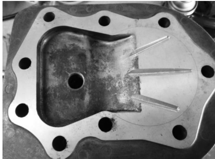
Head surfaced with Singh grooves milled in
