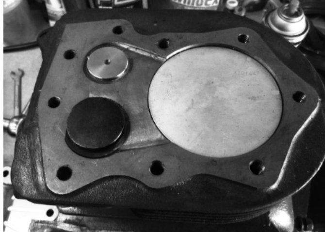
Piston and valves installed
