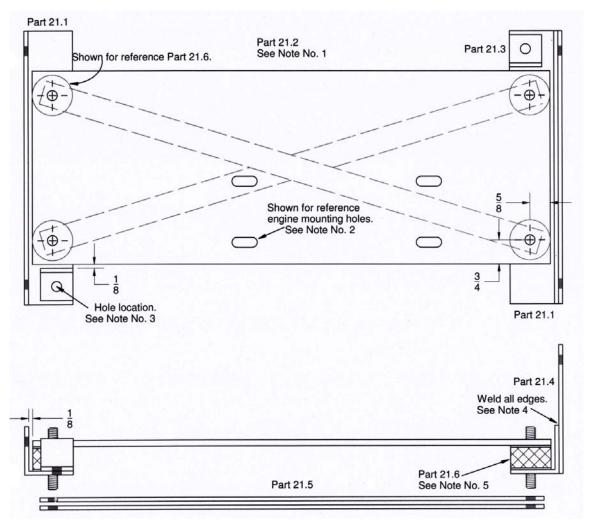
Here's a shrunken version of Randy's CAD drawing from the Club Special plans, showing the mounting plate. Adapting it for use in a Model 1, 2 or 3 should be no big trick.
