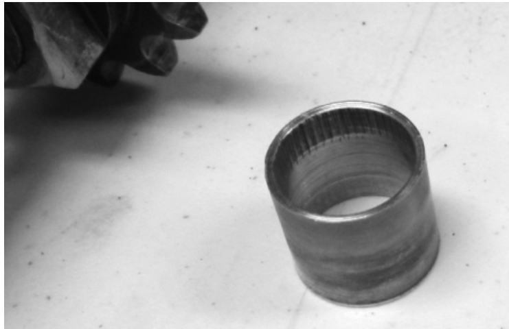
Nearly half this bushing has worn away
