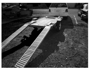
Those ramps shown above are cheap steel ones. A 2x6 can be trimmed to slide inside serving as ramp extenders when needed.
