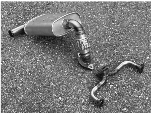
Completed muffler (top) and header (bottom) sections
