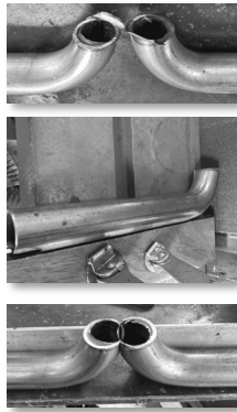
Forming the "siamesed" header joint
