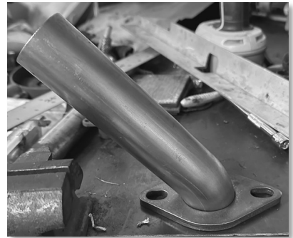
45-degree elbow for muffler assembly before trimming
