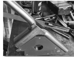
45-degree elbow for muffler assembly before trimming
