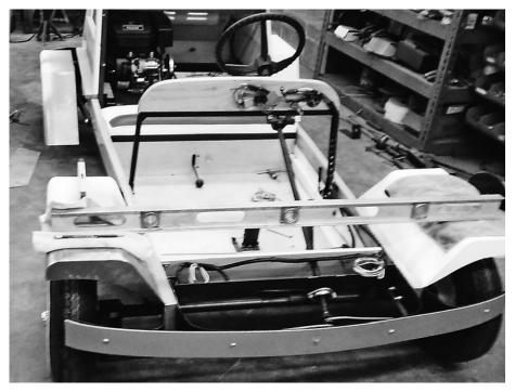
Note the bumper shown here is a flat aluminum bar. A second narrower strip was added for increased stiffening and improved appearance.
